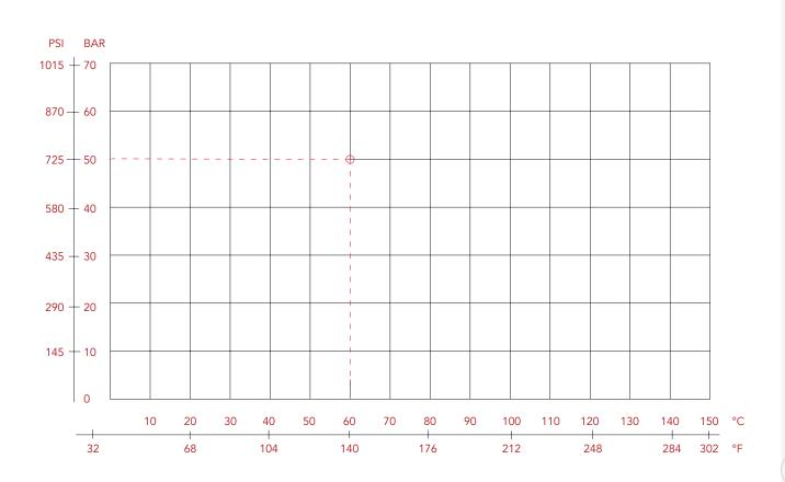
NB: Maximum working temperature for gas: +60  $^{\circ}\text{C}$  The working pressure for gas is from 0 to 5 bar.
